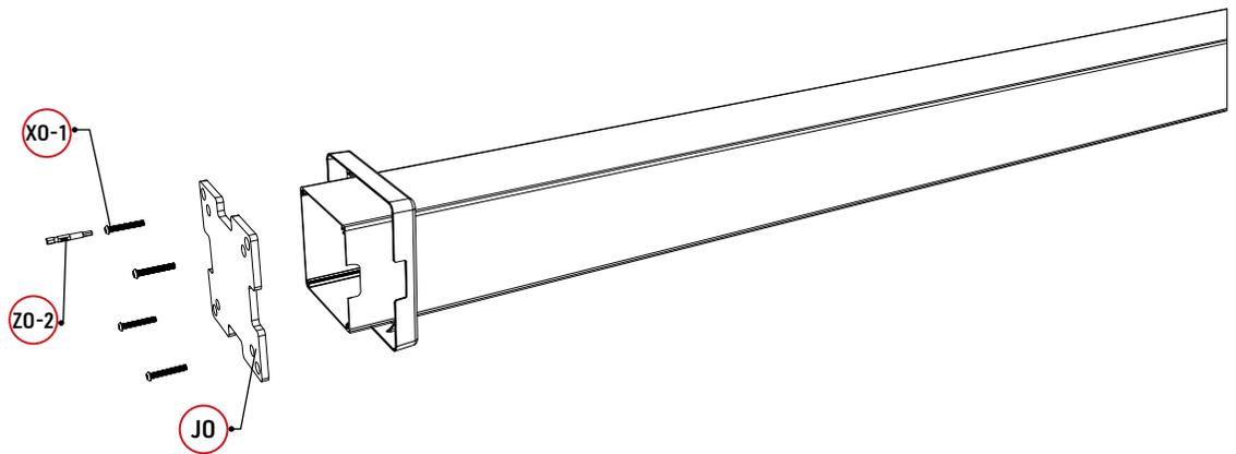
3. Using the pistol drill to fix screws on the plate, please tighten screws with the spanner.
