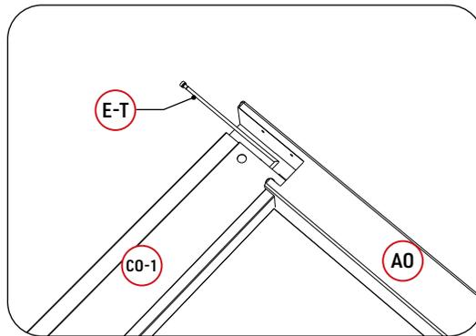
Using the pistol drill to fix screws on the post, then tighten screws with the spanner.
