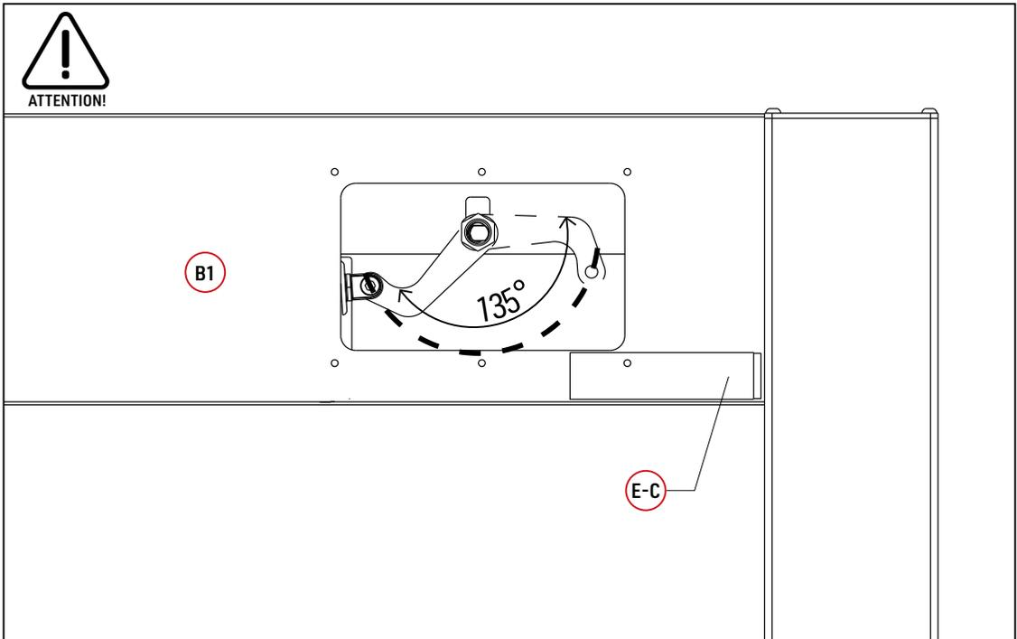
1. Install other louvers on the beam and make the louver flat
