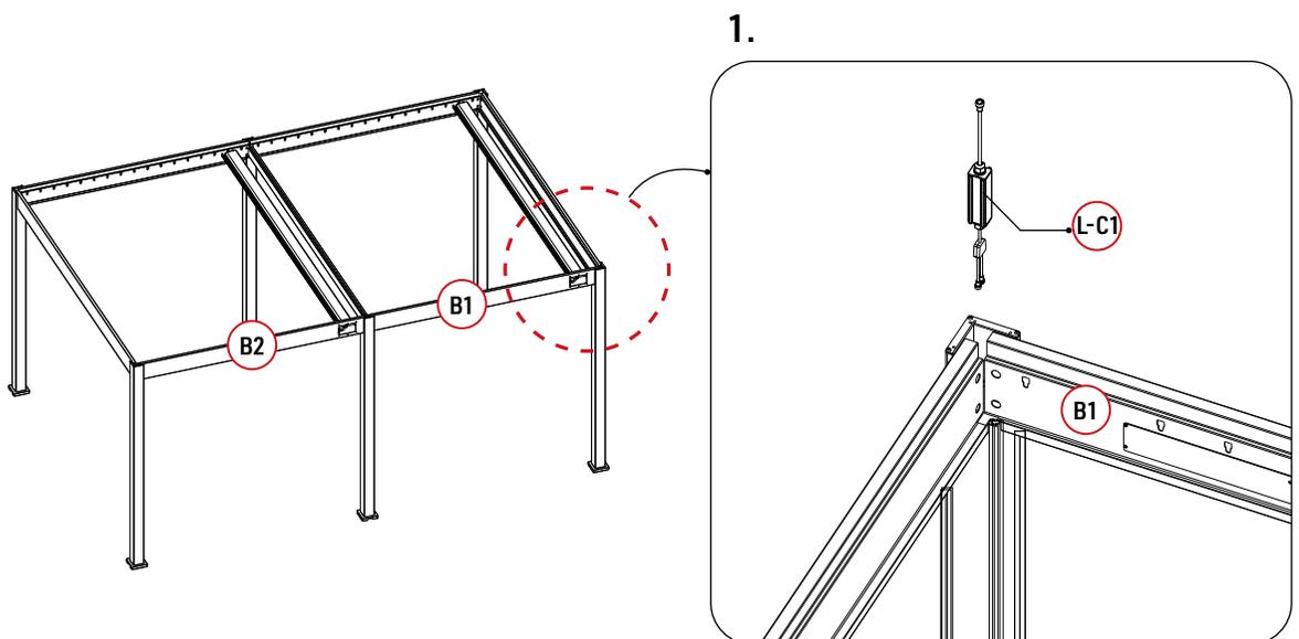
Please note that the Input End of the LED controller should be in the upward direction while the Output End should be in the downward direction.
