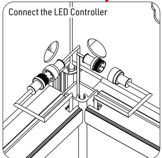
Plug in the power when the connection are well prepared, press bottom 'LED SWITCH' to turn on/off the LED lights.
