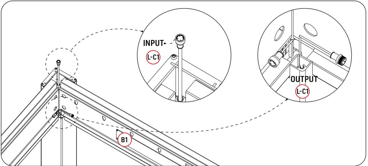
Connect the Input line of the LED controller(L-C1) with the 2# LED of the Controller(E-C).
