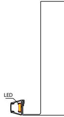
Put the output line of the LED controller(L-C1) into the cavity of the post.
