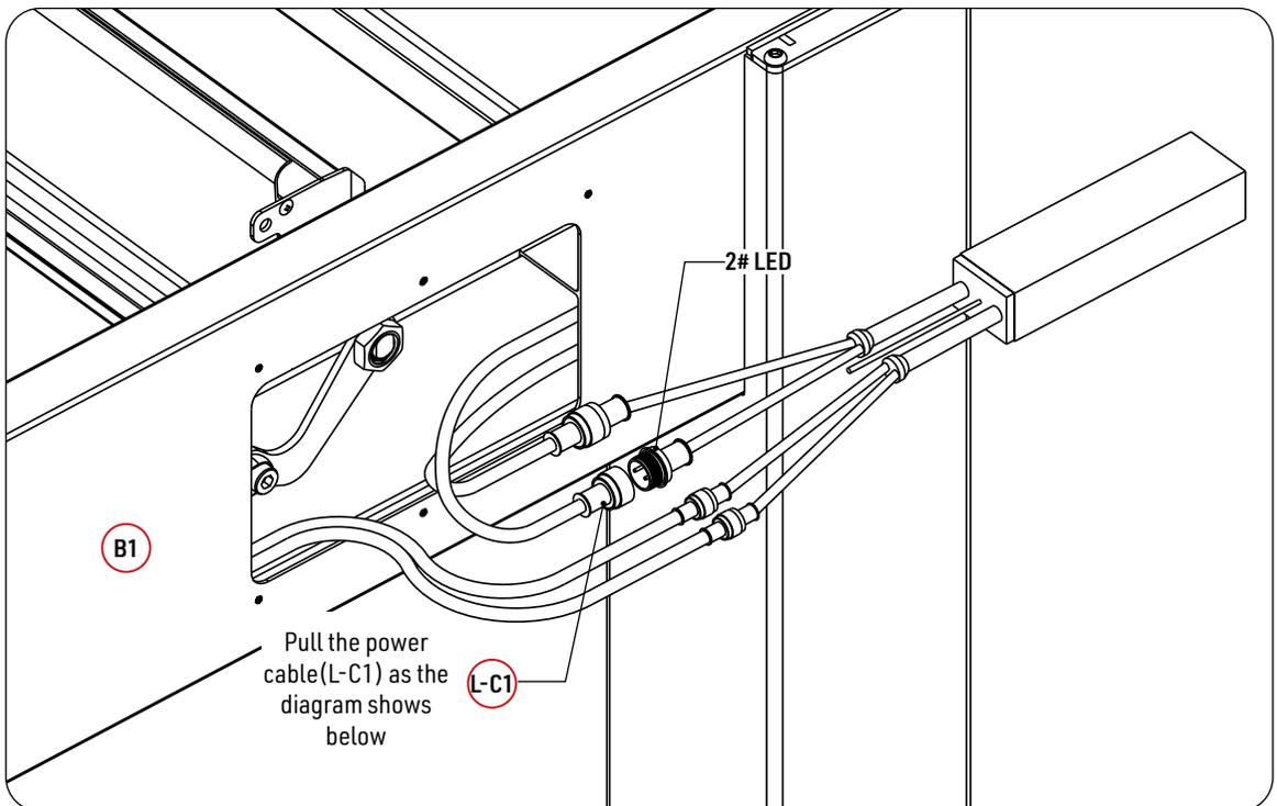
Install all LED strip in series, then connect the two ends of the LED strip with the two output line of the LED Controller(L-C1)
